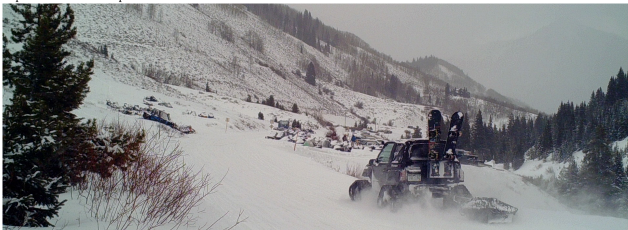
Figure 3. An example of over-snow vehicle progression. Pictured is a Geo Tracker which has been modified through the addition of Side by Side/UTV tracks for the purpose of shuttling owners to and from Irwin, CO.
