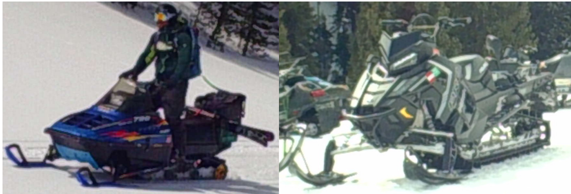
Figures 1 and 2. Shown for contrast is a mid-1990's Polaris RMK700 snowmobile (above, left); once the pinnacle of snowmobile technology. Today these are noteworthy because of their "lead sled" moniker which illustrates the machines disproportionate power to weight rating, a direct byproduct being the undesirable characteristic of sinking in snow. Capabilities are not enhanced by the short track and paddle (~133x1.25"), conventional equipment of the day. Beside the lead sled (above, right) is essentially a modern incarnation of the same machine; this 2017 Polaris RMK800 is inordinately more effective for backcountry travel. Note the elongated track (163x2.6") and increased suspension travel (illustrated by the distance from the snow to the bottom of the machine/tunnel). Numerous improvements over the years have made these machines far more capable than their predecessors.
