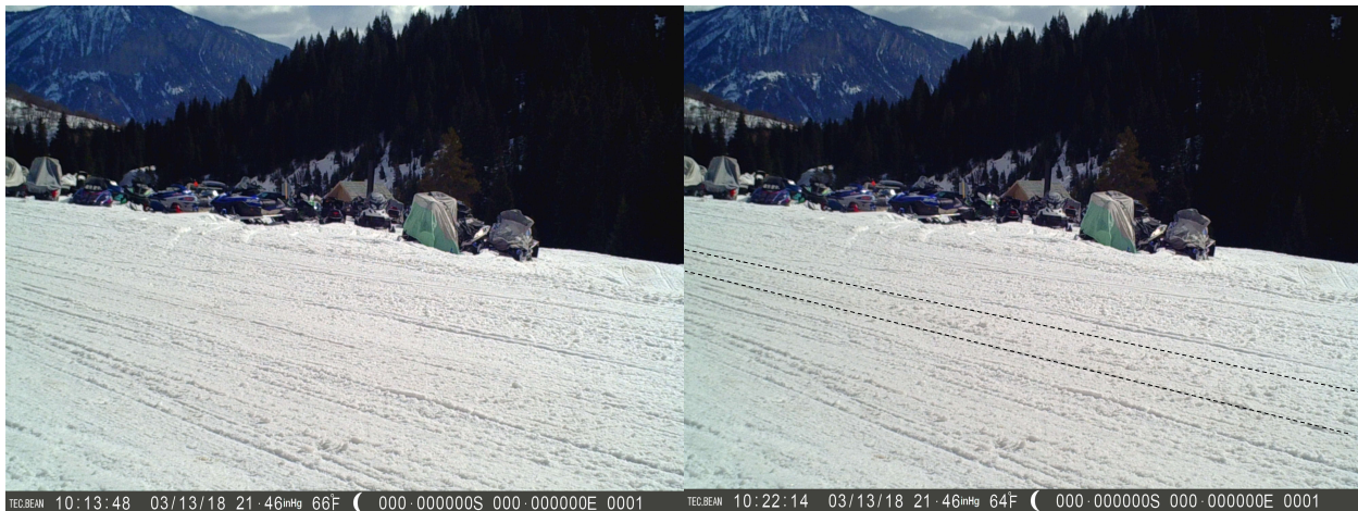
Figures 11 & 12. The above pictures illustrate an example of the camera shutter speed issue discussed in the text. Note the time, date, and additional snowmobile tracks (indicated in the picture on the right with black dotted lines). These pictures were taken contiguously.
